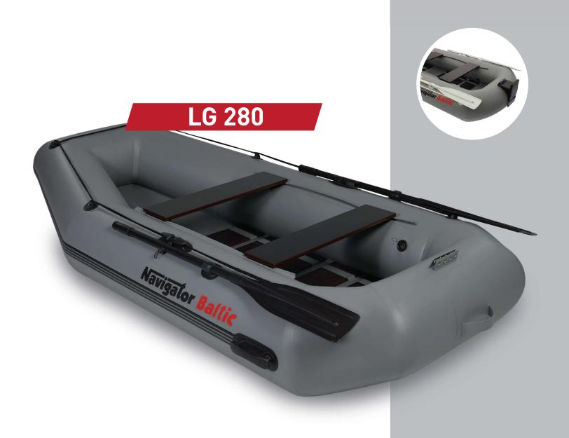
All LG series boats are equipped with the plate for mounting a hinged transom (a transom is not included in standard features).
