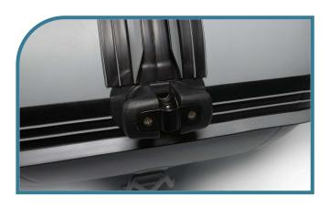
An anchor roller is designed to facilitate dropping and heaving the anchor.
